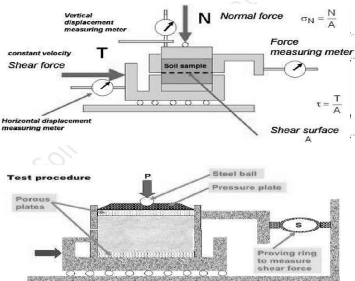
**Step 1: Apply a vertical load to the specimen and wait for consolidation**
